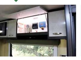
With such legendary durability off the beaten track, it only makes sense that the Elite Goulburn Off Roader brings impressive free camp power options to match. As standard you'll find the van fitted with twin 105AGM deep cycle batteries, a generator box, a 130W solar panel, a VITRON battery charger and a MPPT solar controller. Whatever power needs you have are well and truly covered by such a substantial investment in comfortable remote living.
